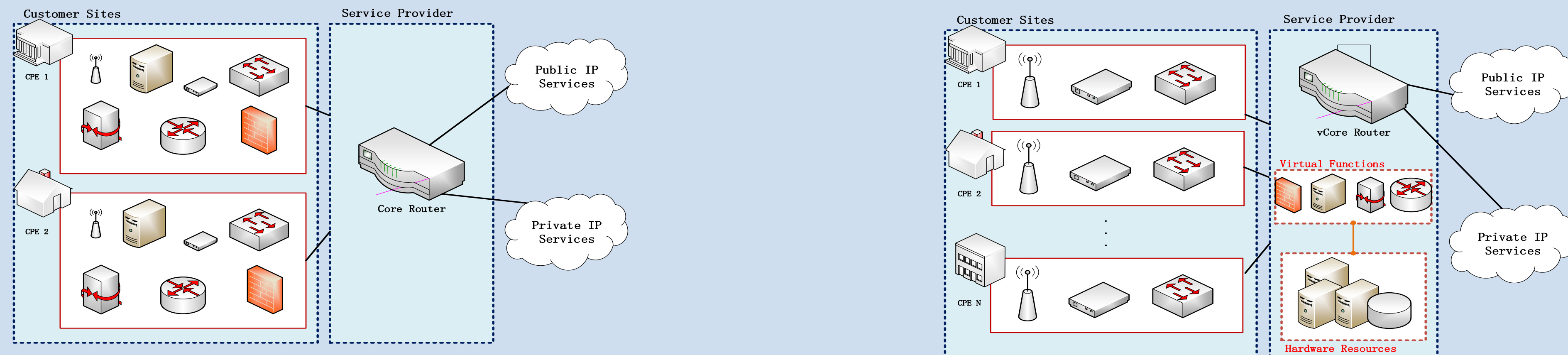
Figure 1. Left side: traditional CPE with ossification issues. Right side: possible CPE with NFV solution.
